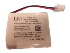
This Li-Ion battery uses a MP176065xlr cell which is ideally suited for applications requiring high energy, long operating life under cycling conditions and offers excellent performance in harsh environments.
